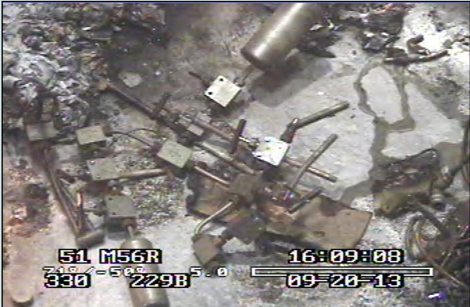
View of North Box Line processing trough after fire event.
